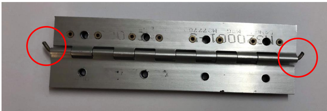
Figure 2. New hinge with correct locking of hinge pin according to HT_ASM_ULS_004_01_02 below (Appendix A)
