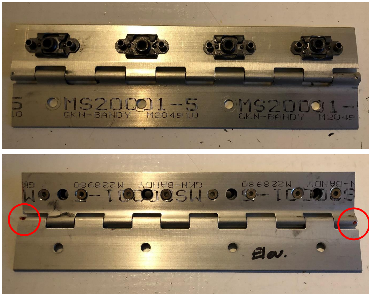
Figure 1. Removed hinge with faulty locking of hinge pin. Area marked that needs to be drilled out (about 5mm)
