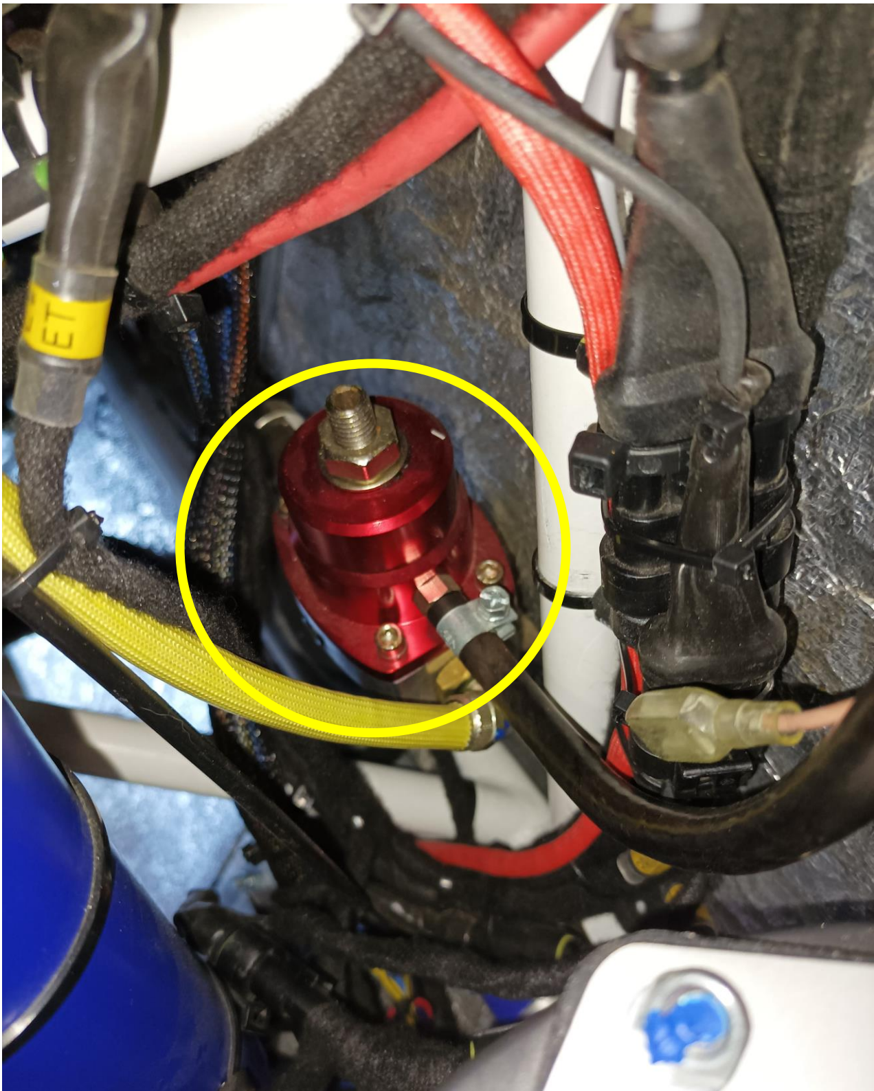
Figure 3. Fuel pressure regulator to be replaced.
