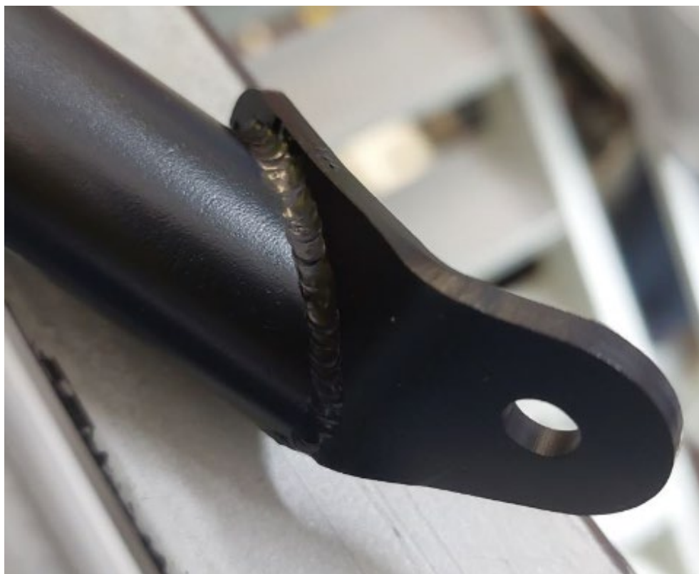
Figure 002 Example of correct welding on the control stick connection rod
