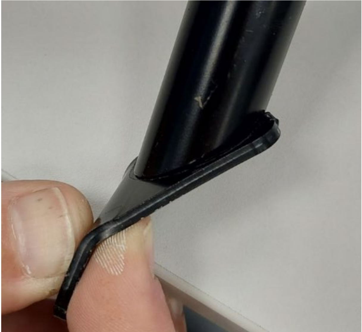
Figure 003 Example of incorrect weld on the control stick connection rod
