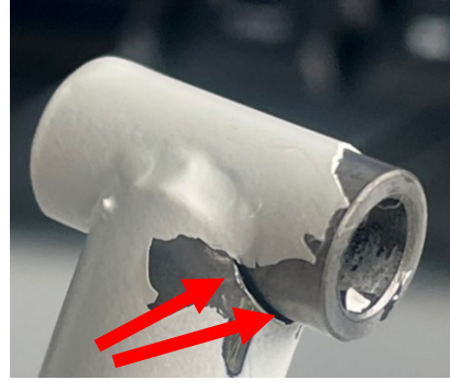
Figure 8 - Weld seams don't cover the entire circumference of the tube, red arrows pointing at the missing weld seams - example with paint partly removed.
