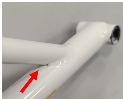
Figure 10 - Another instance of a missing weld seam at the tube corner contact point .
